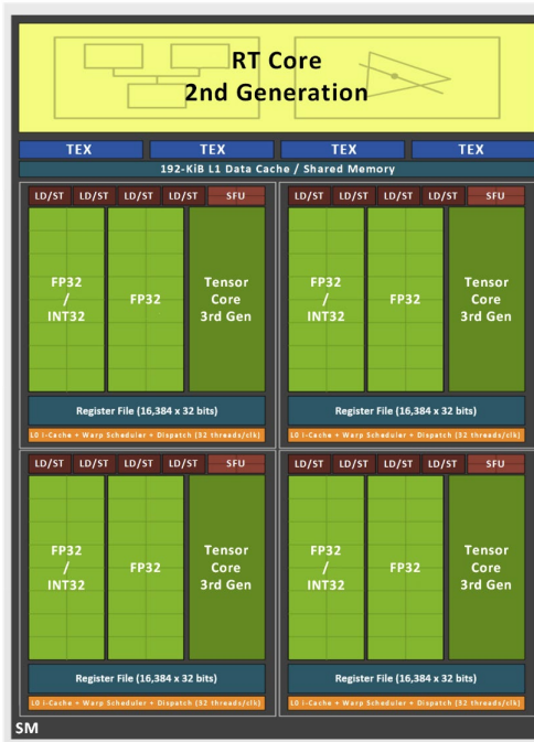
Figure 13 – Ampere Streaming Multiprocessor block diagram (from [2])
